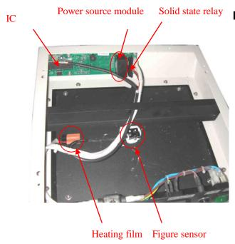
Maintenance: Use Philip screwdriver to loosen the six screw in the base-plate, and take down the base-plate, and there will be a power source module on the main board in the instrument as it shows on the picture. And take down the power source module from the main board by hand, if it is difficult to take down the power source module with hand, you can use the flat apparatus as flat
